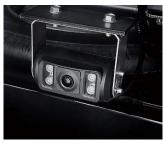
The new eCanter comes standard with a wide-angle rearview camera. A monitor located in the position of the overhead mirror allows the driver to check behind the vehicle.
